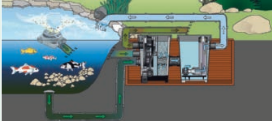
Schematic diagram: ProfiClear Premium Compact-M gravity fed system
